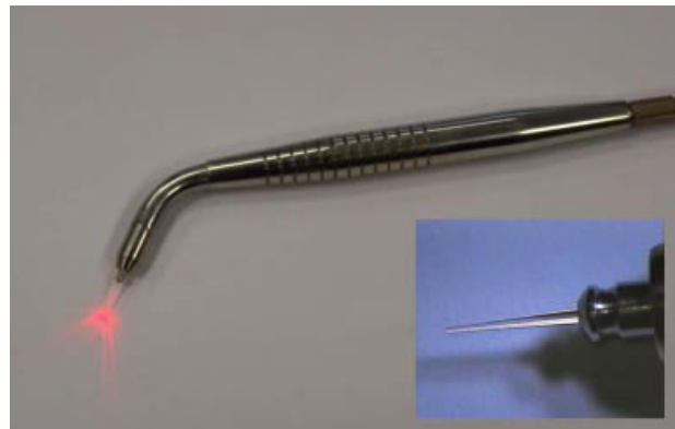
Fig. 3. New laser handpiece with conically shaped fiber tip, adapted to the diode laser (the radially out coupled light of the red pilot beam is visible); small figure: Grinded and polished sapphire taper ( l = 12 mm, \varnothing_{\text{in}} = 800 \mu\text{m} , \varnothing_{\text{out}} = 200 \mu\text{m} ).
