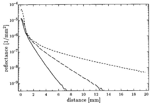
**Fig. 7.** Spatially resolved diffuse reflectance measured for chicken breast (short-dashed curve), bovine muscle (long-dashed curve) and bovine liver (solid curve) *ex vivo* at 633 nm. No polarizers were used.
