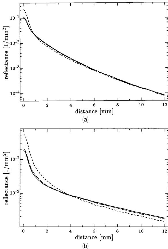
Fig. 4. Tests of the similarity relation that use Monte Carlo simulations for spatially resolved reflectance. For (a),  $\mu_s' = 1.0 \text{ mm}^{-1}$ ,  $\mu_a = 0.01 \text{ mm}^{-1}$ , and  $g = 0$  (short-dashed curve), 0.8 (long-dashed curve), 0.95 (solid curve). The incident beam was 0.4 mm in diameter. Conditions were the same for (b) except that  $\mu_s' = 0.2 \text{ mm}^{-1}$ .
