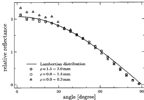
Fig. 2. Angular distribution of diffusely reflected light as calculated by Monte Carlo simulation for  $\mu_s' = 1.0 \text{ mm}^{-1}$ ,  $\mu_a = 0.01 \text{ mm}^{-1}$ ,  $g = 0.9$ , and an incident pencil beam. Results are shown for three radial bins: 0–1.5 mm, 1.5–3.0 mm, and 0–0.3 mm. The Lambertian distribution is also shown as a solid curve. Deviation from the Lambertian distribution is greatest for regions close to the source.
