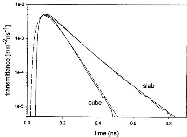
Fig. 4. Comparison of the time-resolved transmittance from a cube ( $l_c = 9$  mm) and from a slab ( $d = 9$  mm) calculated with the diffusion theory (dashed curves) with Monte Carlo simulations (solid curves).
