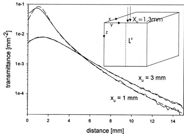
Fig. 6. Comparison of the spatially-resolved transmittance from the lateral side of a cube ( $l_c = 41$  mm) calculated by the diffusion theory (dashed curves) with Monte Carlo simulations (solid curves). The light beam is incident 1 mm and 3 mm away from the edge of the cube's top side. The dashed line in the inset gives the location of the measurement of the transmittance,  $L^s$ .
