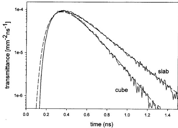
Fig. 3. Comparison of the time-resolved transmittance from a cube ( $l_c = 19$  mm) and from a slab ( $d = 19$  mm) calculated with the diffusion theory (dashed curves) with Monte Carlo simulations (solid curves).
