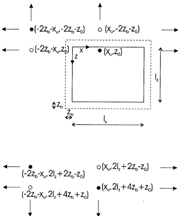
Fig. 2. Two-dimensional arrangement of the positive (solid circles) and negative (open circles) sources to fulfill the extrapolated boundary conditions. The four sources shown at the top of the figure are those for  $l=0, n=0$ , and the four sources at the bottom are those for  $l=0, n=1$ ; see Eq. (5). The extrapolated boundaries are depicted by dashed lines. The arrows indicate that the point sources in each row are continued to infinity.
