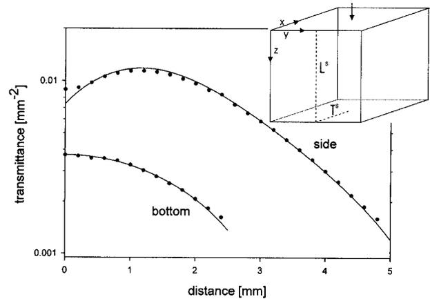
Fig. 5. Comparison of the spatially resolved transmittance from the bottom and the lateral side of a cube ( $l_c = 9$  mm) calculated by the diffusion theory (solid curves) with Monte Carlo simulations (circles). The light beam is incident on the middle of the cube's top side. The dashed lines in the inset give the location of the measurement of the transmittance from the lateral side,  $L^s$ , and from the bottom side,  $T^b$ .
