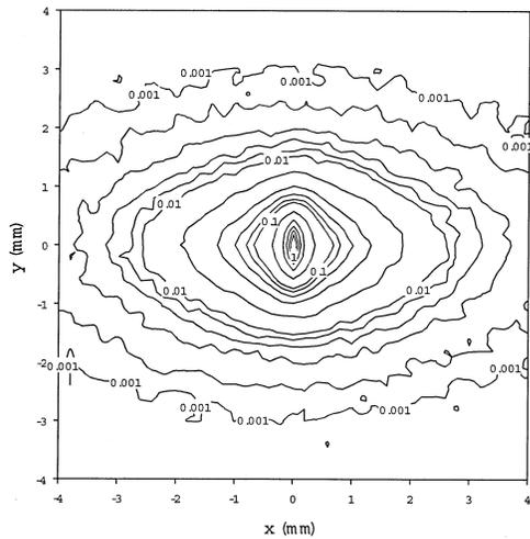
Fig. 3.  $R(x, y)$  pattern ( $\text{mm}^{-2}$ ) obtained from Monte Carlo simulations of a semi-infinite turbid medium containing isotropic scatterers and cylinders along the  $x$  axis with  $\Delta\eta = 0$ .
