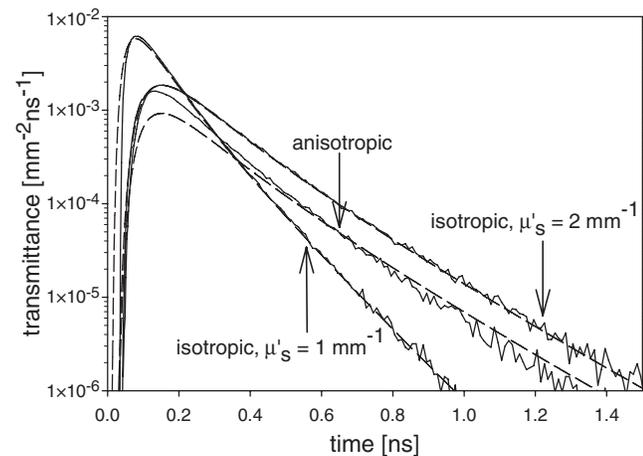
FIG. 3.  $T(x = 0$  mm,  $y = 0$  mm,  $t$ ) calculated with MCt (solid lines) and solutions of the diffusion theory (dashed line). The detection area in the simulations was  $\Delta x \Delta y = 1$  mm $^2$ .
