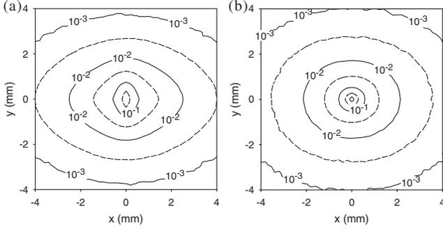
FIG. 1. Spatially resolved reflectance  $R(x, y)$  (unit:  $\text{mm}^{-2}$ ) calculated with (a) MCc and with (b) MCt.
