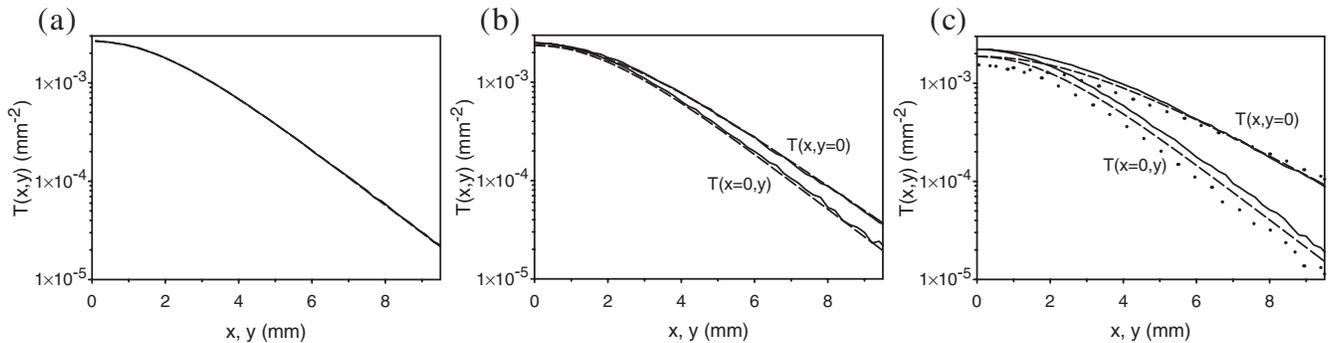
FIG. 2. (a) Spatially resolved transmission along the  $x$  and  $y$  directions for a slab with  $\mu'_{sx} = \mu'_{sy} = \mu'_{sz} = 2 \text{ mm}^{-1}$ . In (b) and (c)  $\mu'_{sx}$  was changed to  $1.6 \text{ mm}^{-1}$  and  $1.0 \text{ mm}^{-1}$ , respectively. Data were calculated with the anisotropic diffusion equation (dashed curves), with MCt (solid curves), and with MCc (dotted curves).
