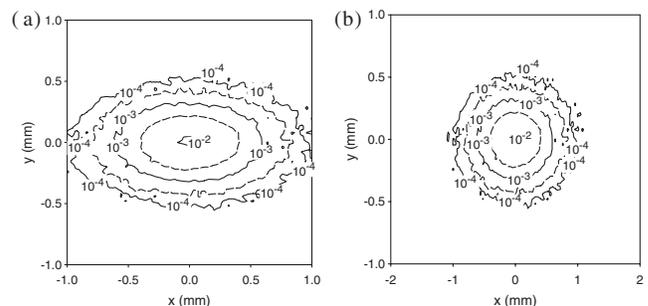
FIG. 4. (a)  $T(x, y)$  (unit: mm $^{-2}$ ) from a slab with  $\mu'_{sx} = 1500$  mm $^{-1}$ ,  $\mu'_{sy} = \mu'_{sz} = 10000$  mm $^{-1}$ ,  $\mu_a = 0.00079$  mm $^{-1}$ ,  $d = 0.31$  mm,  $n_m = 1.4$  and  $n_o = 1.0$ ; (b) same as (a), but the  $x$  axis was multiplied by 2.
